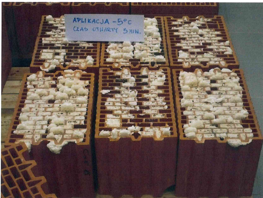
Picture 6. General view of selected specimens after the test (clay blocks more filled with polyurethane are the lower parts of the specimen)
