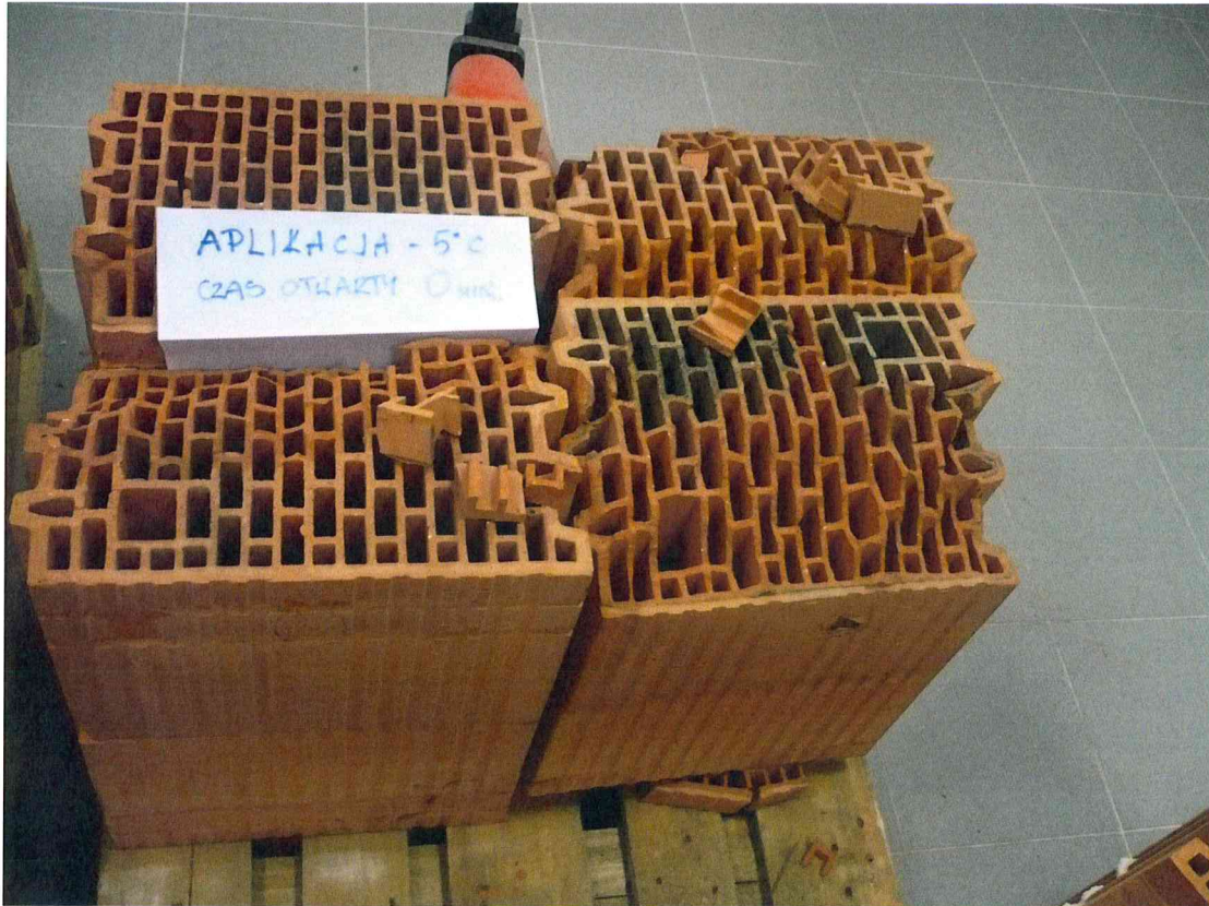
Picture 5. View of specimens, which were destroyed within clay block
