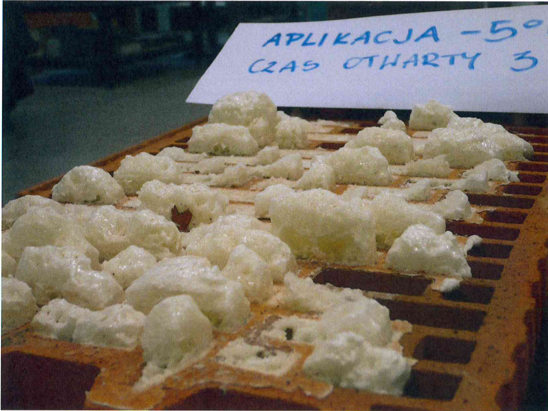
Picture 7. Specimen after testing - polyurethane on bracket surface was applied on
